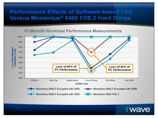
What this slide shows is (SWA, SWB, SWC are Software Encryption Products) the loss of performance is indicated.
