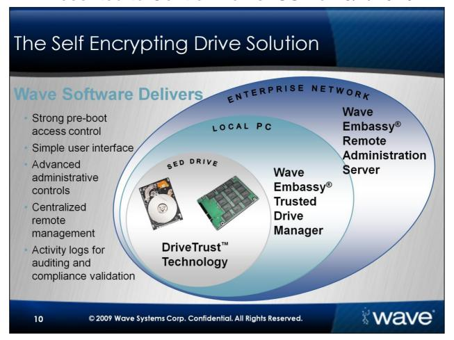
This slide shows the hardware and Wave software components at the Enterprise Level and the Local PC Level. This explains the architecture, with hardware at the heart of it. The bullets describe several features that are very critical to any kind of enterprise deployment.
